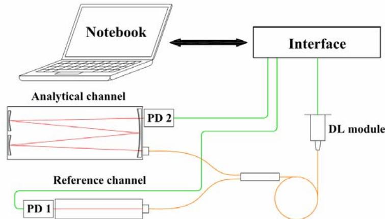
**Figure 2: Trace HF molecule concentration detector general schematic**
